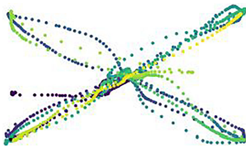
Fig. 7 Visualization of the mouse usage behavior of a sample participant in the drag-and-drop task. The rectangular frame represents the computer screen. The dots represent single mouse data points. Mouse movement data points are chronologically ordered from purple to yellow. Mouse clicks are represented by black dots
